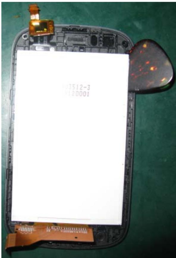
2). Use the hot wind gun in temperature 130°C, air level 3-4, height 5-10mm, blow the TP for about 5 to 10 minutes and use plastic flake to pry up the TP remove it from face shell.
