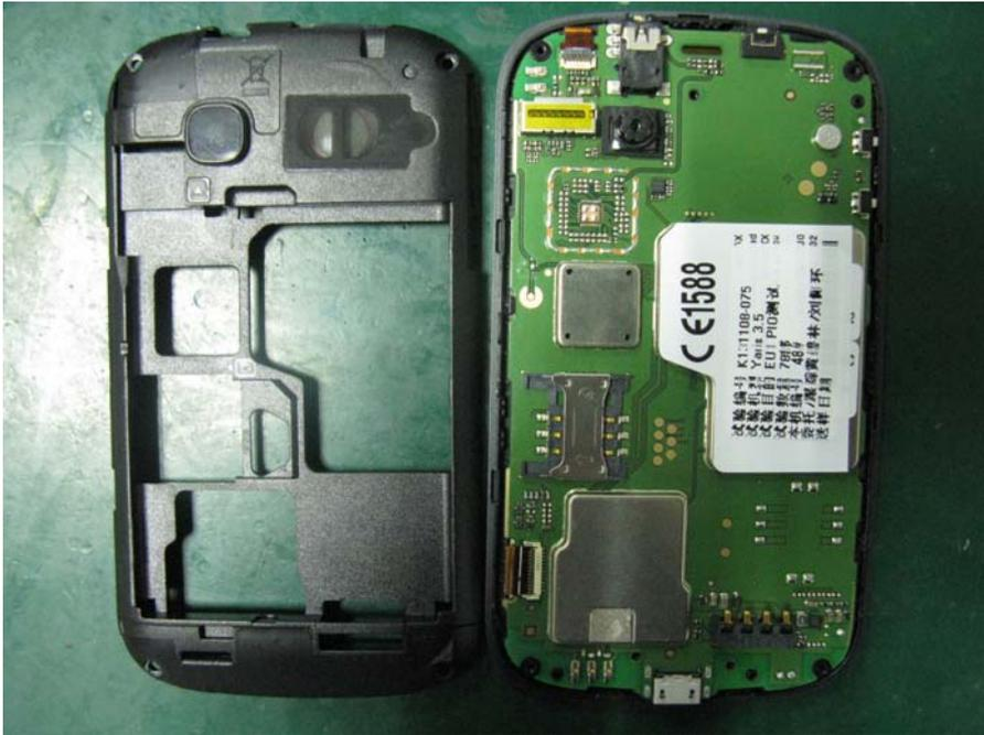
**NOTE:** The furnished back cover can't be reused if any of the buckles is deformed or damaged.
